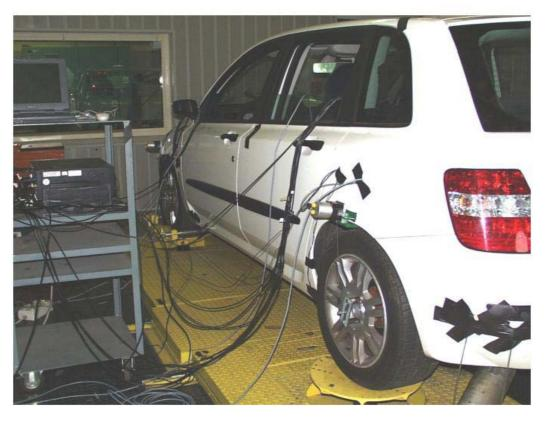
• Measurements are performed on a four-poster test bench of FIAT-Elasis Research Center.
